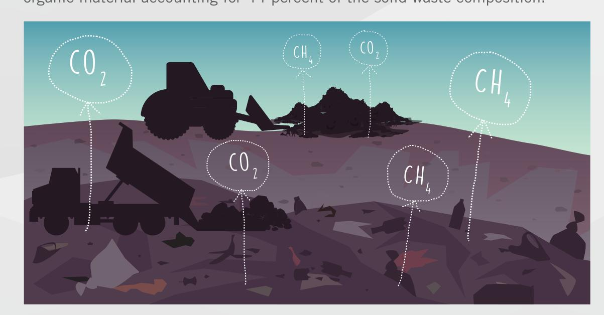
The bacterial decomposition of organic material and oxidation of solid waste produces landfill gas, which is composed of methane (CH<sub>4</sub>) and carbon dioxide (CO<sub>2</sub>), potent GHGs that contribute to the global climate crisis. Without incentives to install landfill gas capture and destruction systems, Argentina's waste sector would continue to experience waste management challenges and produce a significant source of methane emissions.
