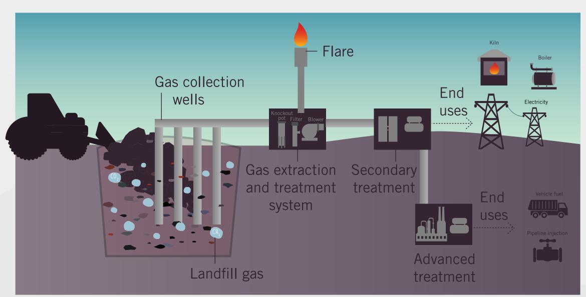
Landfill gas collection and destruction systems consist of technologies that enable or enhance the collection of landfill gas (such as wells, pipes, blowers, and caps) and convey it either to a destruction technology (such as flares) or to an energy recovery system (such as engines, generators, or boilers). The project achieves methane reductions to benefit the climate and produces high-quality carbon credits that can be sold in the carbon market, helping to offset the system costs.
